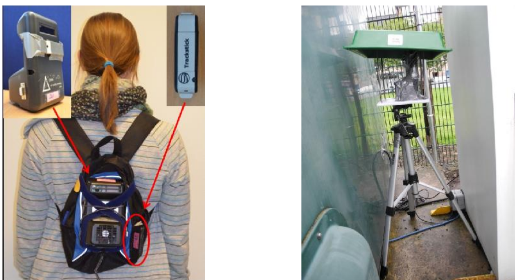
Fig. 1. Illustration of the monitoring pack for mobile measurements (left) and the rain cover and tripod for stationary outdoor deployment (right)
