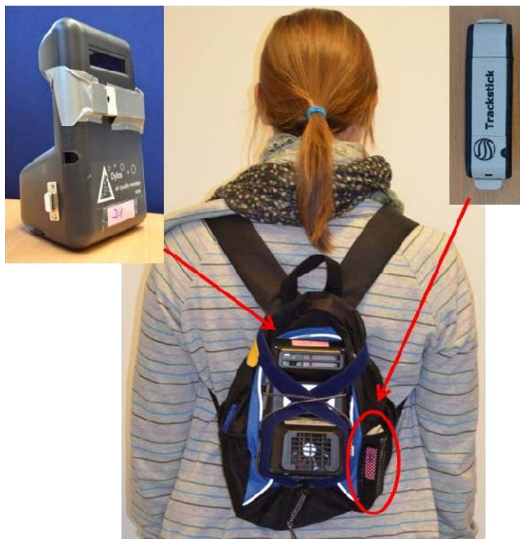
Figure 3.1. The monitoring pack - the Dylos instrument is strapped onto the backpack with the back exposed to the air. To avoid the interface buttons being pushed accidentally, we put a protective plastic cover over it. A hole drilled into the plastic allows reaching the on/off button with a pen for example. The exposed design of the backpack restricts its outdoor use to dry weather conditions.
